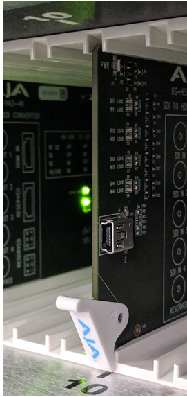
Figure 15. Partially Inserted Card with Unlocked Plastic Tab
