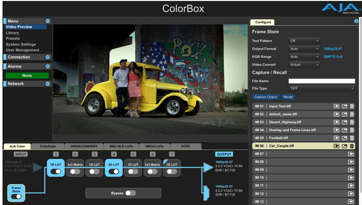
Figure 22. AJA Color Pipeline Example, with Frame Store On
