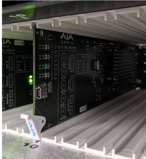
Figure 10. Partially Inserted Card with Unlocked Plastic Tab
