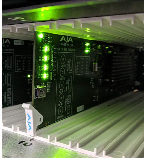
Figure 11. Fully Inserted Card with Locked Plastic Tab
