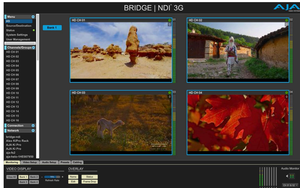
Figure 42. Viewing only Bank 1, 4 HD Channels
