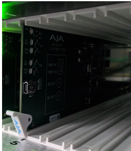
Figure 7. Partially Inserted Card with Unlocked Plastic Tab
