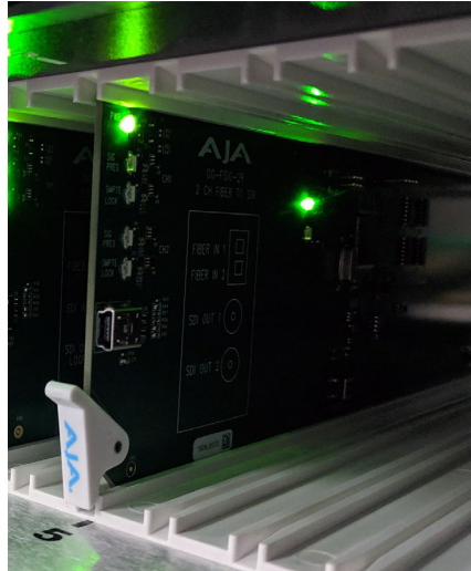
Figure 8. Fully Inserted Card with Locked Plastic Tab
