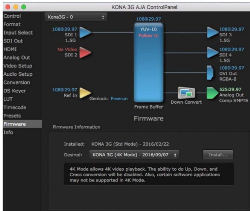
Figure 39. AJA Control Panel, Firmware Screen (Changeover to 4K)
