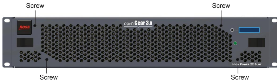
Figure 3.6 OG-3-FR Series Frame — Faceplate Screws Location
