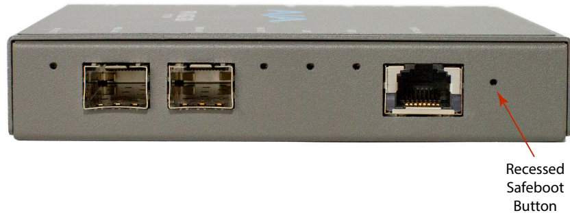
Figure 39. Location of recessed safeboot button
