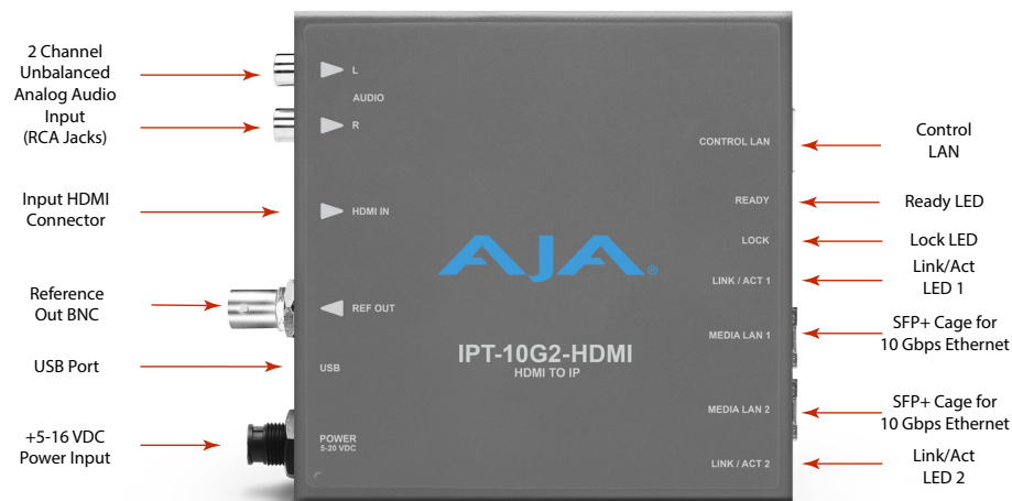
Figure 4. IPT-10G2-HDMI Connections
