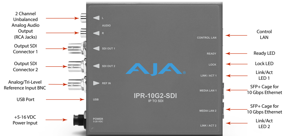
Figure 6. IPR-10G2-SDI Connections
