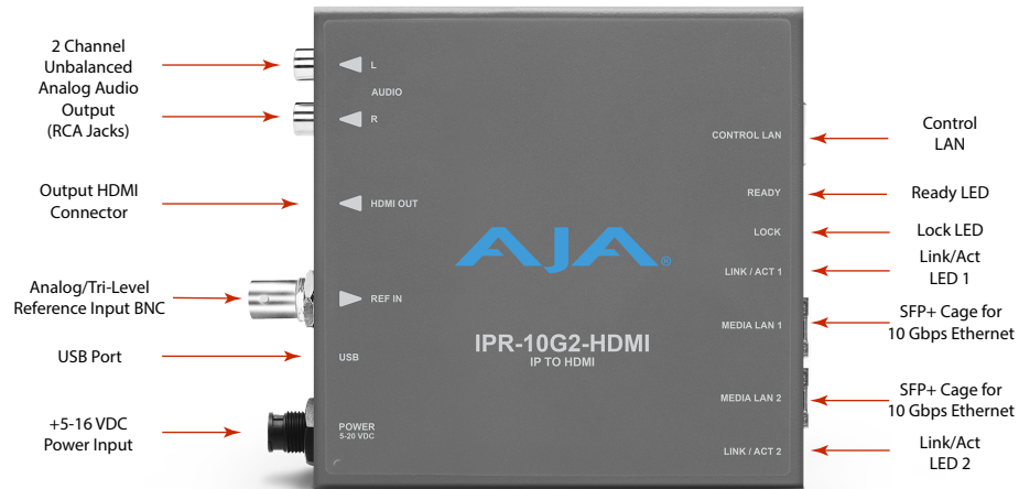
Figure 8. IPR-10G2-HDMI Connections
