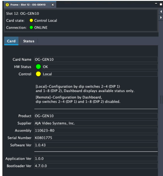
Figure 5. Local Control Specified
