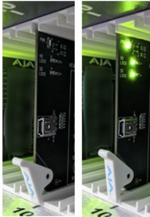
Figure 9. Partially Inserted (Left) versus Fully Inserted (Right) Front Card
