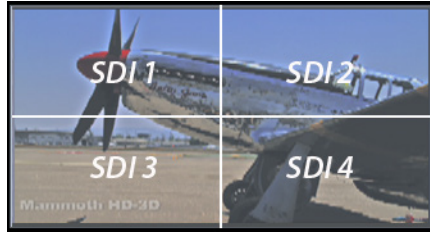
Figure 7. Mapping of Quad SDI Outputs
