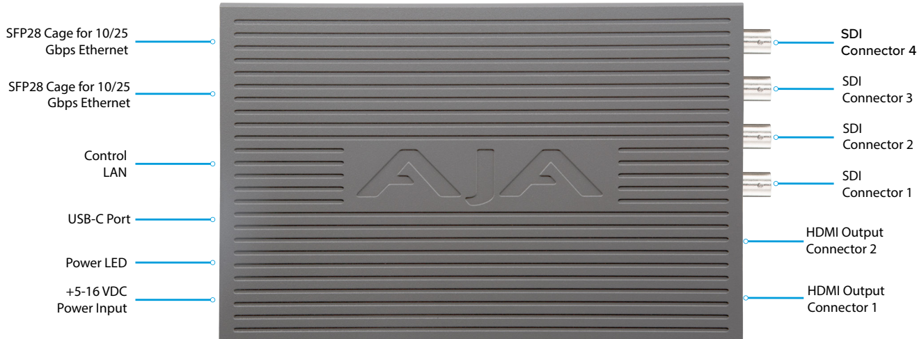
Figure 1. IP25-R Connections, Top View
