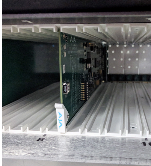
Figure 5. Fully Inserted Card with Locked Plastic Tab
