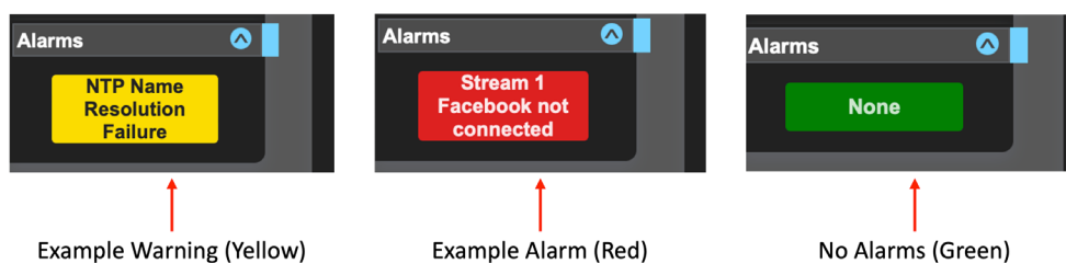
Figure 8. Example HELO Plus Alarm Panes, showing a Warning, an Alarm and None
