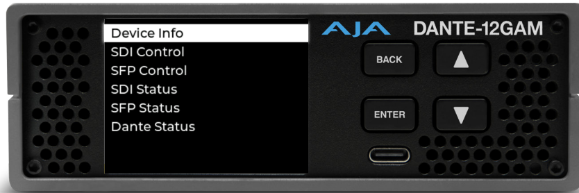
Figure 48. DANTE-12GAM Front Panel Display showing Home Screen
