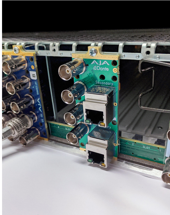
Figure 7. Rear Card Inserted Into Frame Seating Slot
