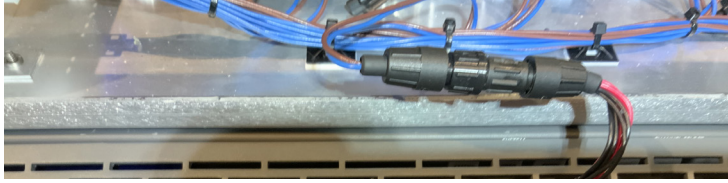
Figure 35. Locate and unplug the Active Faceplate DC power connector
