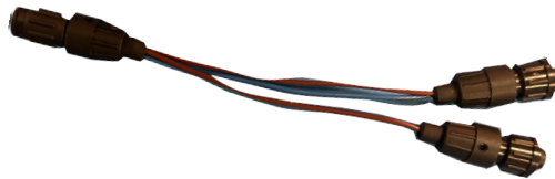
Figure 42. Y-Cable added to DC Power Harness for stacked FiDO expansion
