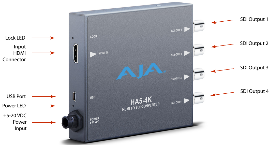
Figure 2. HA5-4K Converter Connections
