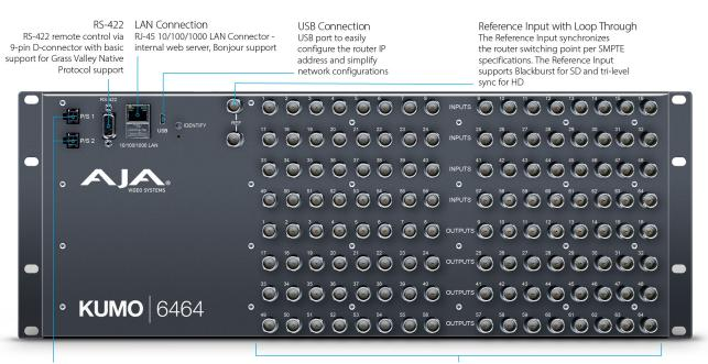
Fully Redundant AC Power Supplies Two independent 12VDC inputs provide safe operations. Power status can be checked from a LAN attached browser 3G-SDI Inputs and Outputs All inputs and outputs, 3G, HD-SDI, or SD-SDI (SMPTE-259/292/424)
