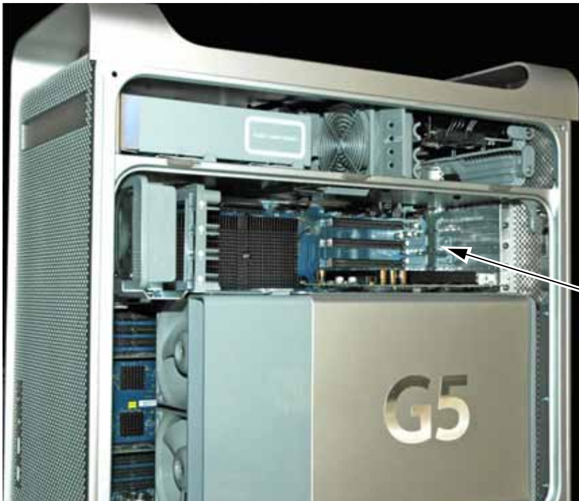
PowerMac G5 Cardcage Access (MacPro card cage differs in appearance)
