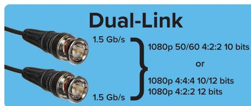
Dual-Link HD-SDI is a single image signal conveyed over two standard 1.5gb HD-SDI cables. This is most often used for 1080p 50/60 video but may also be used for 1080p 24/25/30 at 4:4:4 color encoding and/or 12 bits.
