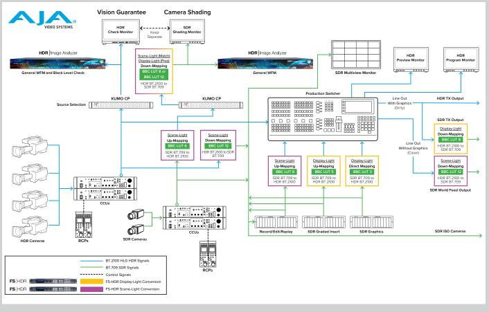
Single Master HDR/SDR Live Production workflow using BBC LUTs with FS-HDR and HDR Image Analyzer.
