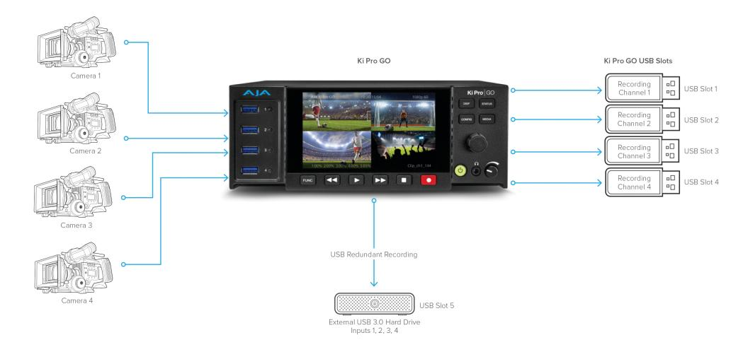
NOTE: v1.5 Firmware provides additional flexibility for user selectable primary and backup recording channels to any port desired
