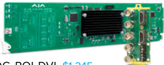
OG-ROI-DVI $1,245 openGear DVI to 3G-SDI Scan Converter with Region of Interest and Frame Synchronizer
