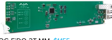
OG-FiDO-2T-MM $1,155 openGear 2-Channel 3G-SDI to Multi-Mode LC Fiber Transmitter
