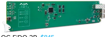
OG-FiDO-2R $845 openGear 2-Channel Single Mode LC Fiber to 3G-SDI Receiver
