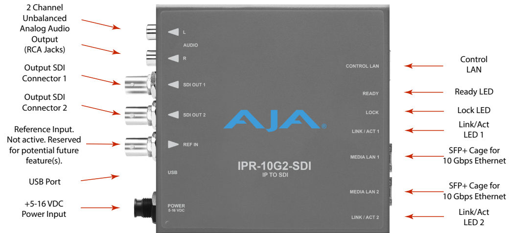
Figure 3. IPR-10G2-SDI Connections
