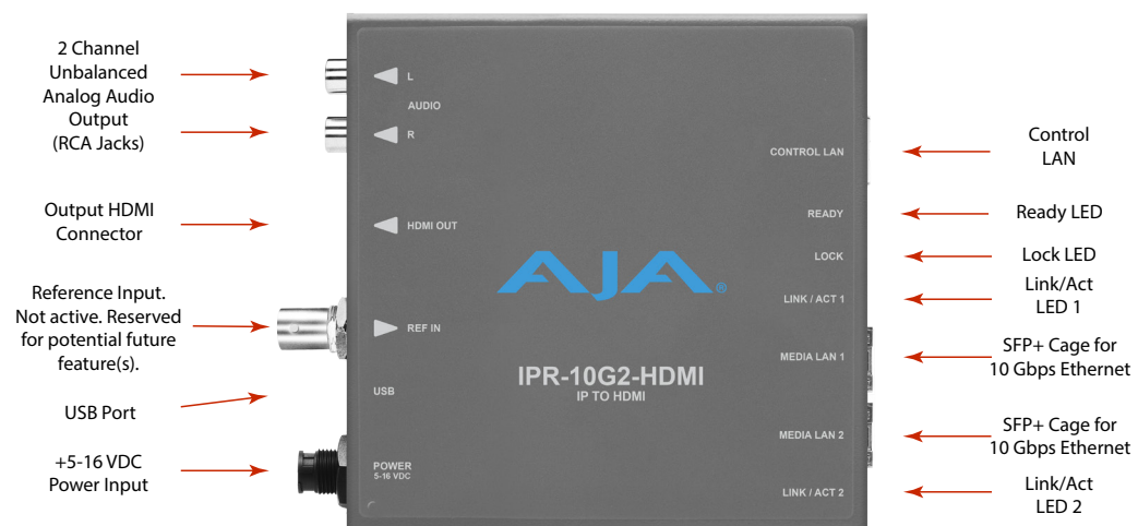
Figure 2. IPR-10G2-HDMI Connections
