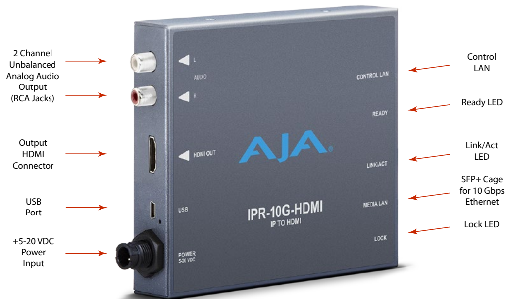
Figure 2. IPR-10G-HDMI Connections
