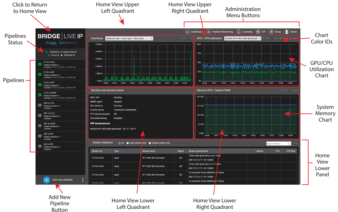
Figure 30. BRIDGE LIVE IP Dashboard Home View
