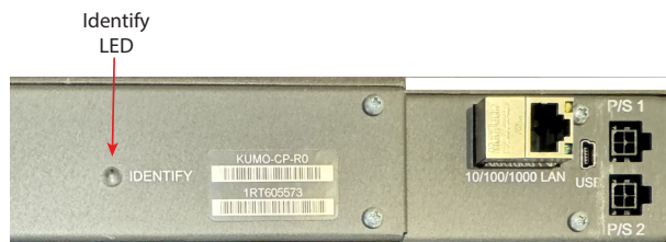
Figure 78. KUMO CP Identify LED Location
