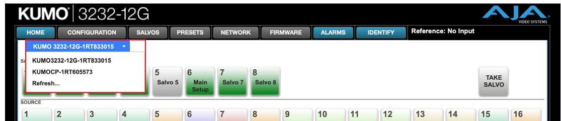
Figure 18. KUMO WebUI Home Screen showing Select Device menu
