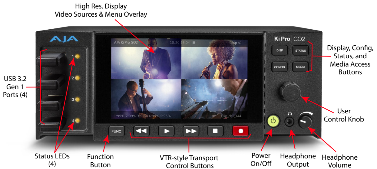
Figure 2. Ki Pro GO2 Front Panel
