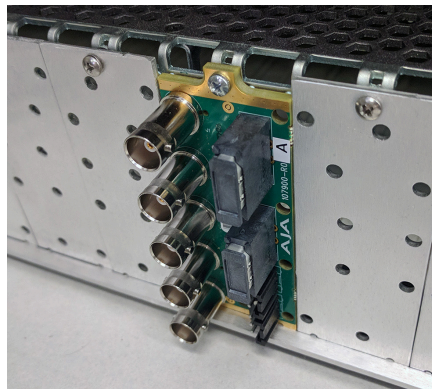
Figure 7. Rear Card Inserted into Frame Seating Slot
