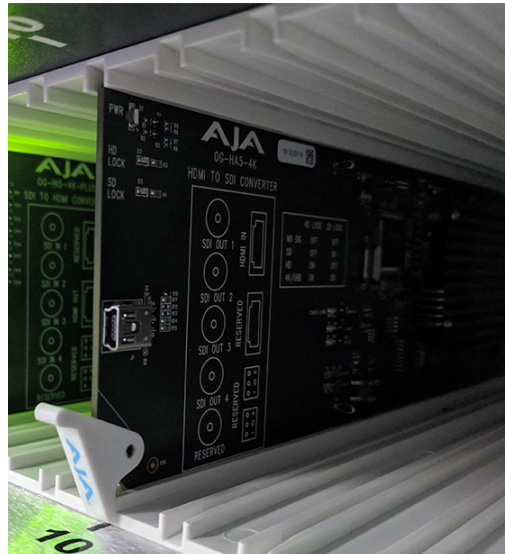
Figure 8. Partially Inserted Card with Unlocked Plastic Tab
