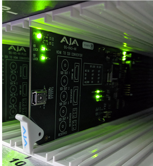
Figure 9. Fully Inserted Card with Locked Plastic Tab
