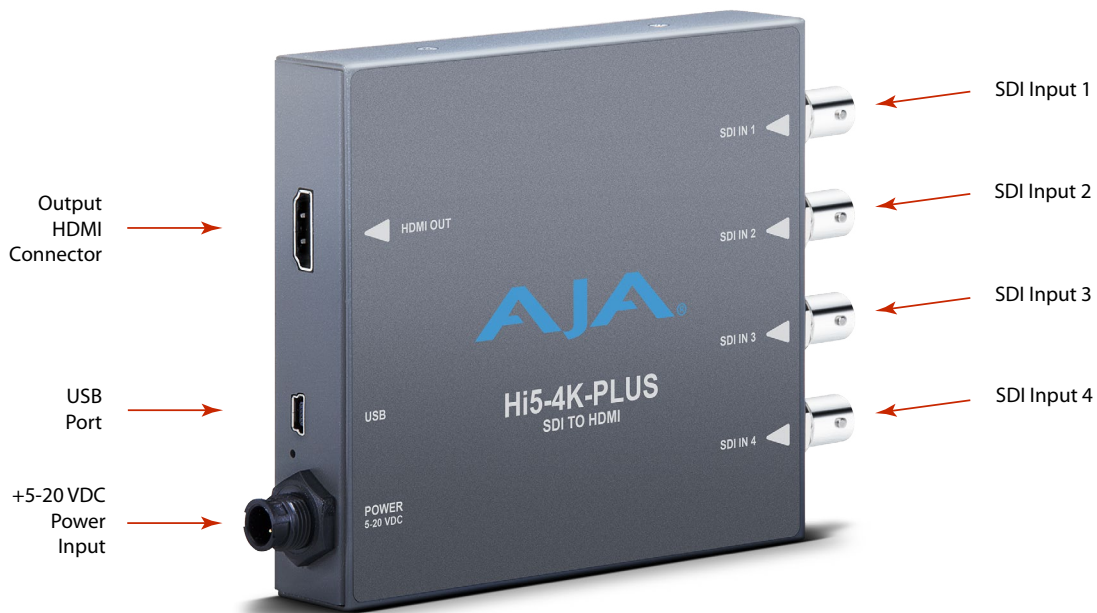
Figure 2. Hi5-4K-Plus Converter Connections
