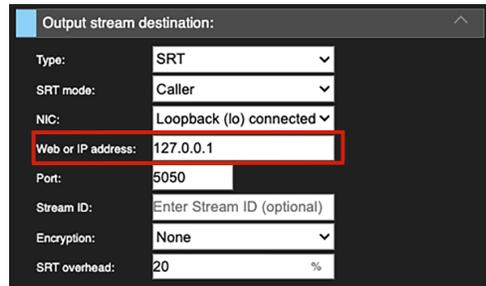
The screenshot shows the 'Output stream destination' configuration panel. The 'Web or IP address' field is highlighted with a red box and contains the value '127.0.0.1'. Other fields include: Type: SRT, SRT mode: Caller, NIC: Loopback (lo) connected, Port: 5050, Stream ID: Enter Stream ID (optional), Encryption: None, and SRT overhead: 20%.
