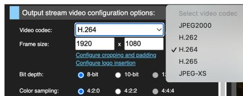
The screenshot shows the 'Output stream video configuration options' dialog. The 'Video codec' dropdown is open, showing a list of options including H.264, which is selected. Other options include JPEG2000, H.262, H.265, and JPEG-XS. The 'Frame size' is set to 1920 x 1080. The 'Bit depth' is set to 8-bit. The 'Color sampling' is set to 4:2:0.
