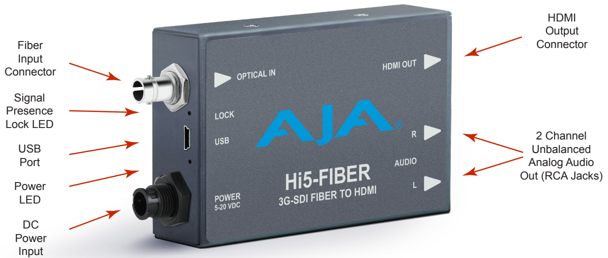
Figure 2. Hi5-Fiber Converter Connections
