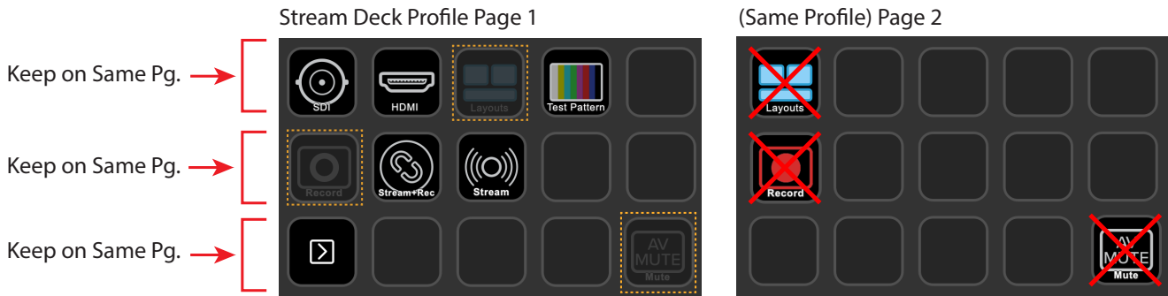
Figure 40. Assign all related Keys in each Action Group to the Same Page
