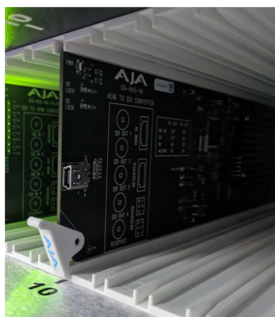
Figure 9. Fully Inserted Card with Locked Plastic Tab
