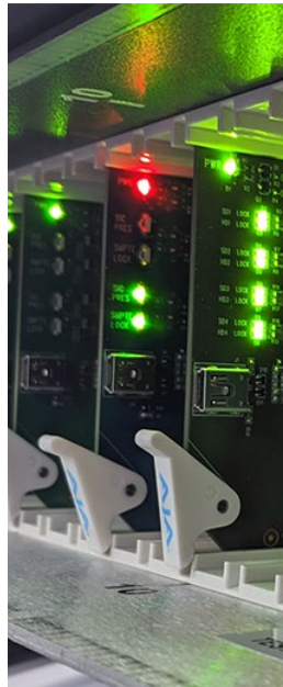
Figure 9. Partially Inserted Card with Unlocked Plastic Tab (Middle)
