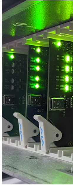
Figure 10. Fully Inserted Card with Locked Plastic Tab (Middle)
