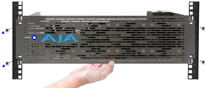
Figure 20. Removing an Active Faceplate
