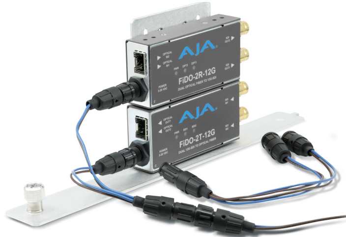
Figure 27. Y-Cable added to DC Power Harness for stacked FiDO expansion
