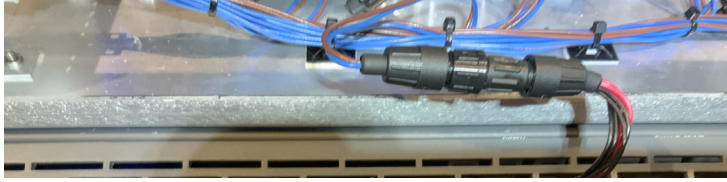
Figure 21. Locate and unplug the Active Faceplate DC power connector
