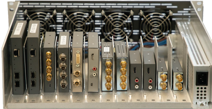
Figure 1. DRM2 with twelve Mini-Converters mounted on Carriers
