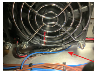
Figure 18. Keep DC power and any other wires from getting inside fan
