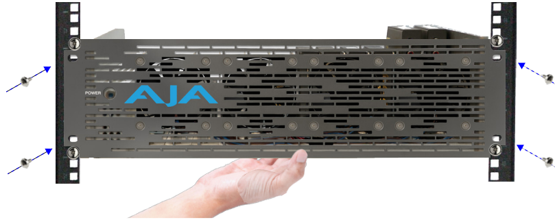
Figure 19. Attaching an Active Faceplate
