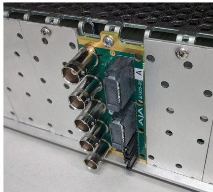
Figure 8. Rear Card Inserted Into Frame Seating Slot
