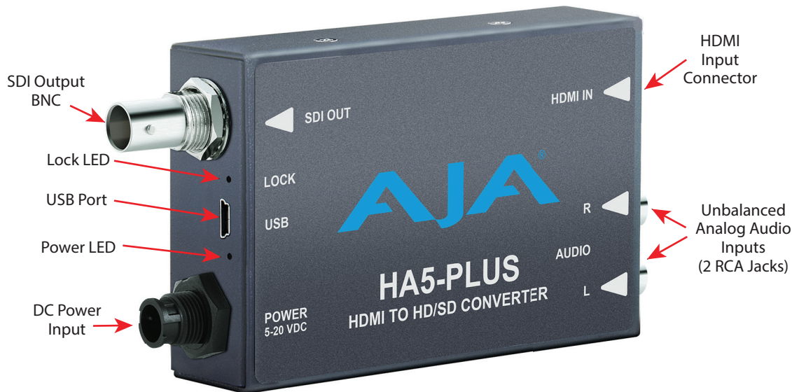
Figure 2. HA5-Plus Mini-Converter
