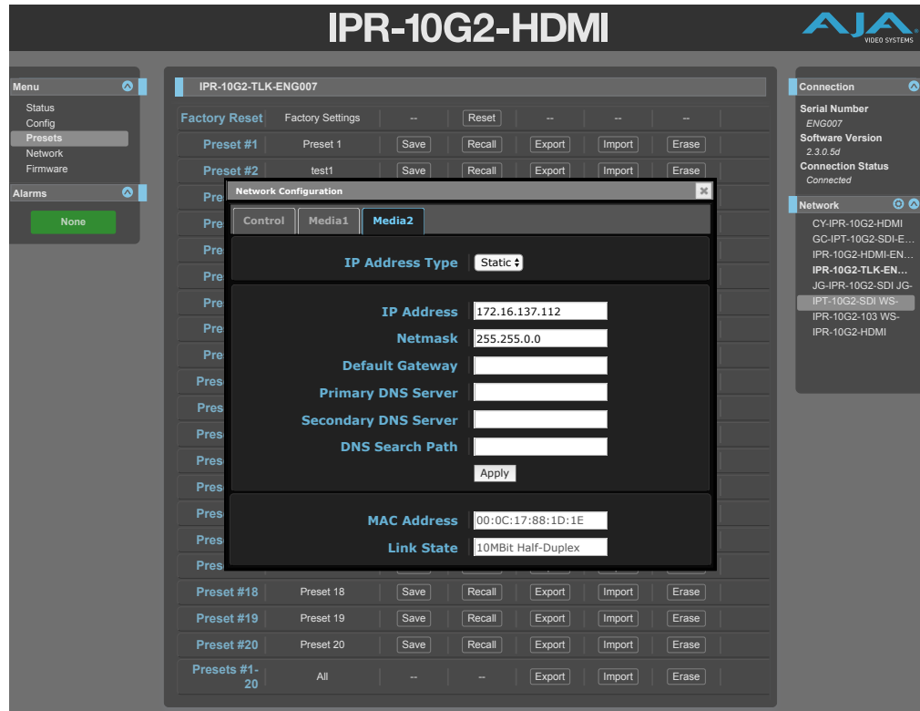
Figure 36. IPR-10G2-HDMI Network Configuration Media 2 Tab
