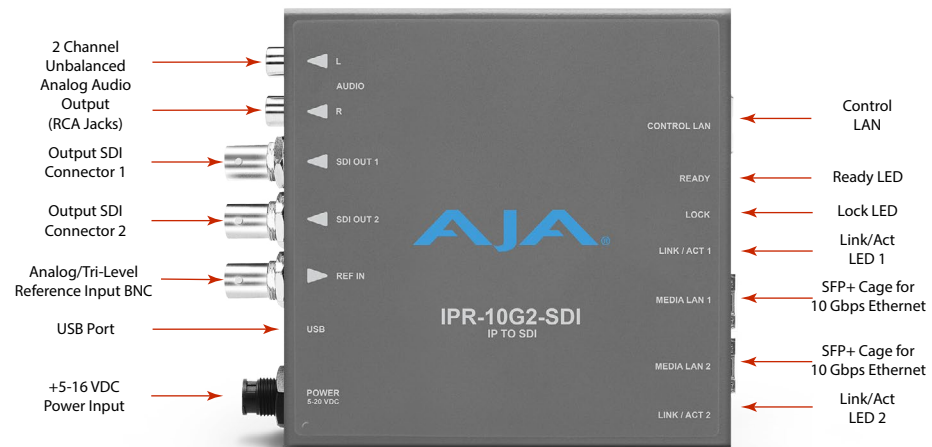
Figure 6. IPR-10G2-SDI Connections
