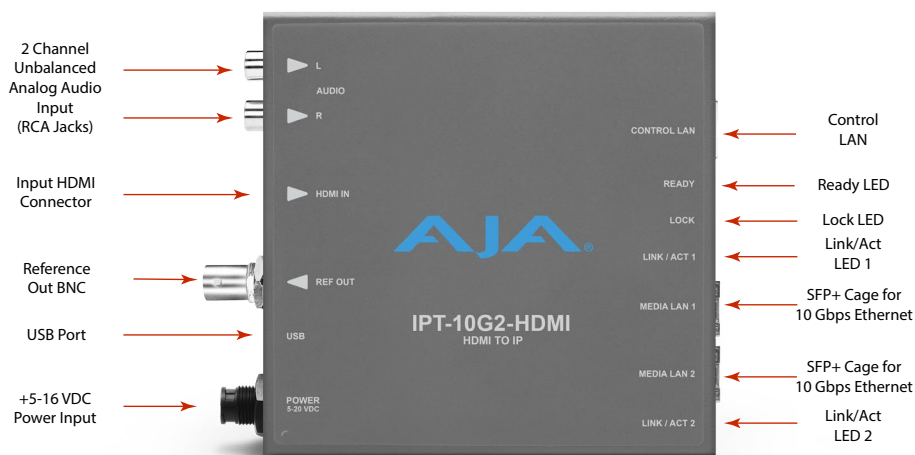
Figure 4. IPT-10G2-HDMI Connections
