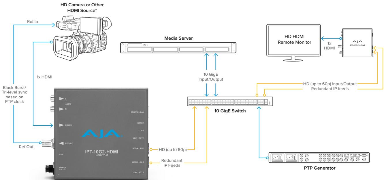
Figure 4. IPT-10G2-HDMI Connections
