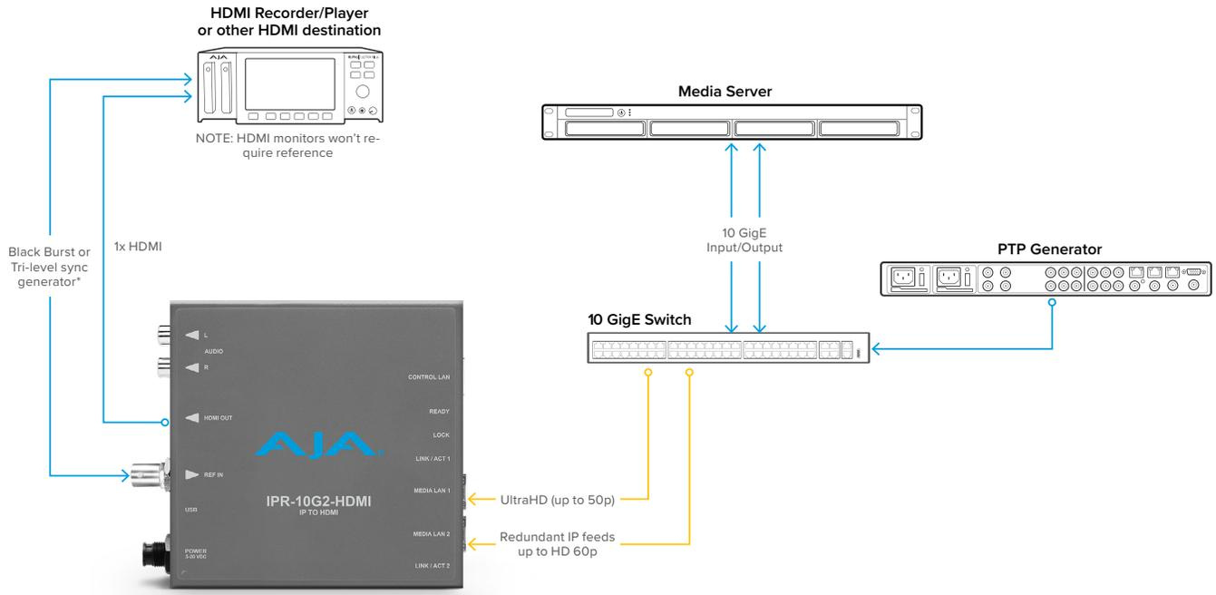
Figure 8. IPR-10G2-HDMI Connections
