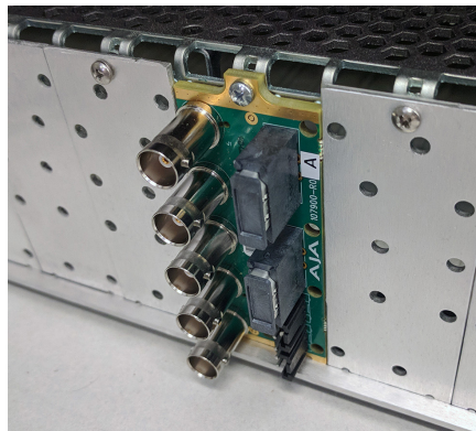
Figure 7. Rear Card Inserted Into Frame Seating Slot
