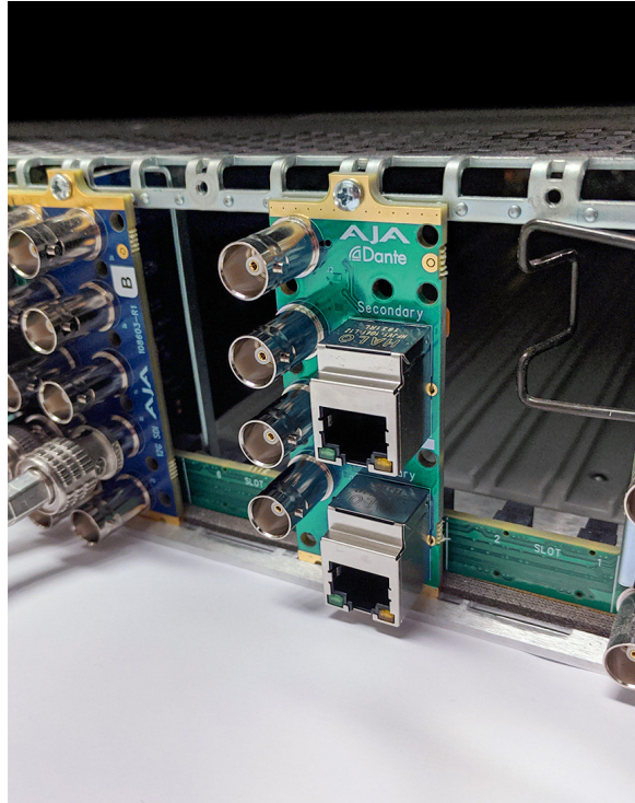
Figure 7. Rear Card Inserted Into Frame Seating Slot
