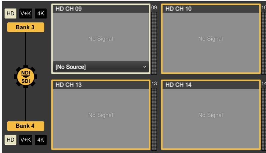
2. Select the drop-down menu. A list of detected NDI sources displays. In this example, eight NDI sources have been detected.
