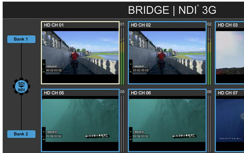
In the example above, all channels of SDI input are being encoded from SDI to NDI. The Bank buttons are blue, as is the outline of each Video Tile, which is the system color for SDI to NDI encoding (SDI In, NDI Out).
