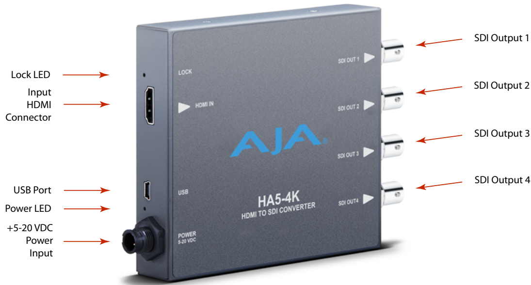
Figure 2. HA5-4K Converter Connections
