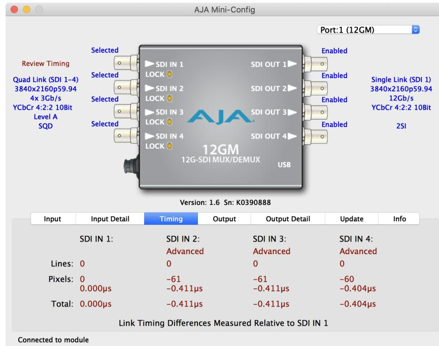
The above Timing Tab Screen shows that links 2, 3, and 4 are equally advanced with respect to link 1 by about 60 pixels. Since all three links are equally advanced, most likely link 1 has an additional function element (piece of processing equipment or additional processing function) which is delaying it 60 lines—so links 2, 3, and 4 appear advanced.
