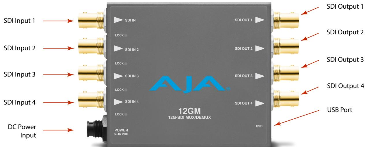
**NOTE:** The LEDs adjacent to each SDI input connector indicate by color the detected signal type. Off is no signal, Green is SD-SDI, Red is HD-SDI, Amber is 3G-SDI, Purple is 6G-SDI, and Blue is 12G-SDI.
