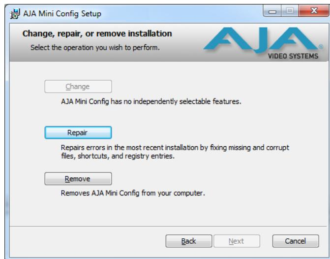
With this screen you can **Repair** (reinstall) or **Remove** (uninstall) AJA Mini-Config on the PC.
