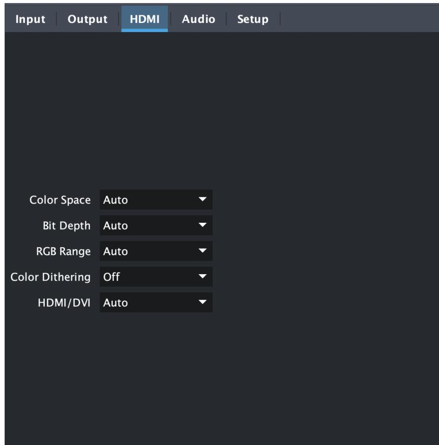
Click on the HDMI tab to view and make changes to the 4K2HD HDMI output settings.
