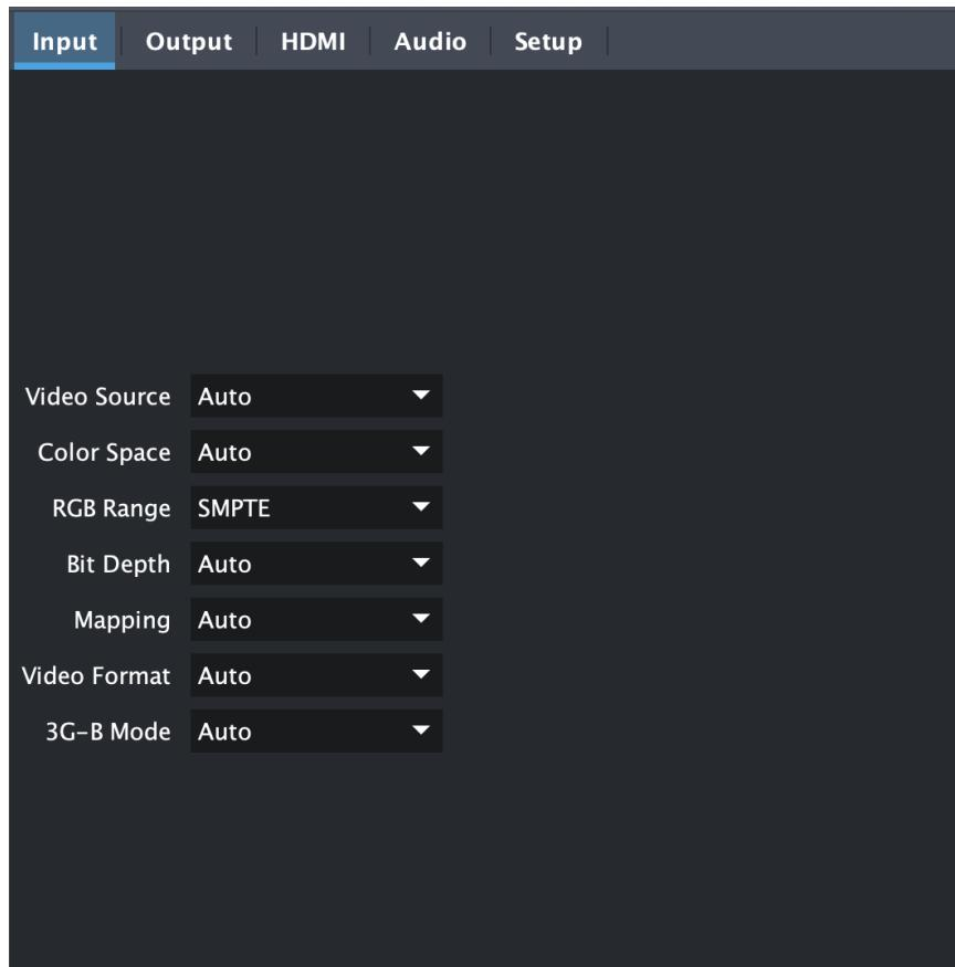
Click on the Input tab to view and make changes to the converter's input settings.
