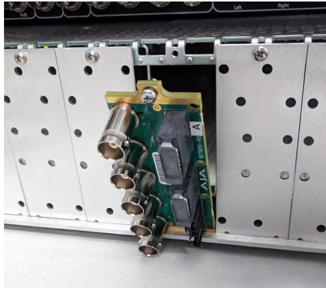
5. Align the top screw of the Rear Card with the screw hole on the top edge of the frame back plane.
