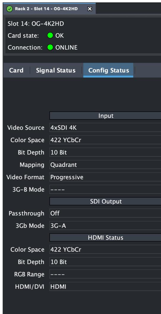
The Config Status tab screen reports the current setting of configuration parameters that are set to **Auto**.
