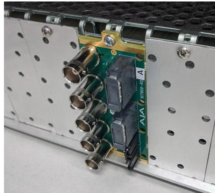
8. Ensure proper frame cooling and ventilation by having all rear frame slots covered with rear modules or blank metal plates if plates are not pre-installed.
