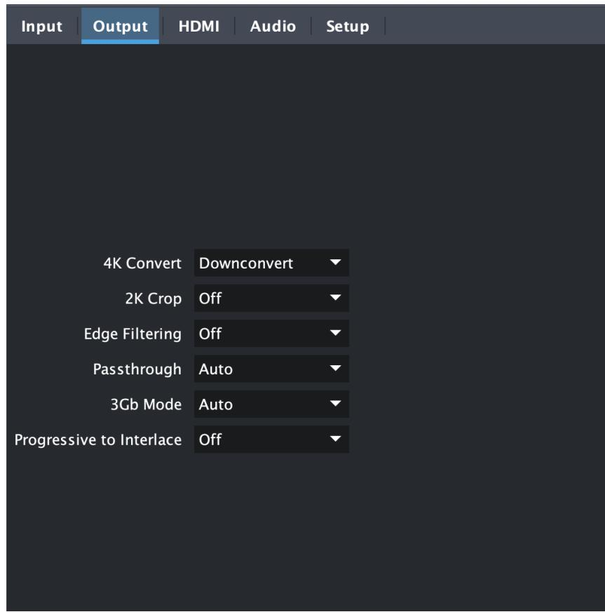
Click on the Output tab to view and make changes to the 4K2HD Output settings. These settings can affect both the HDMI and SDI outputs.
