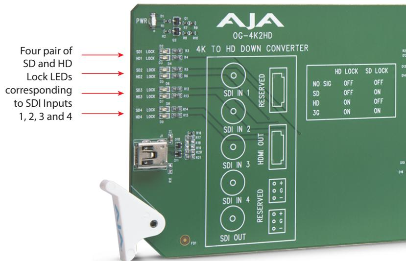
Table 1. The meaning of the behaviors of the lights for each pair of SD and HD Lock LEDs.
