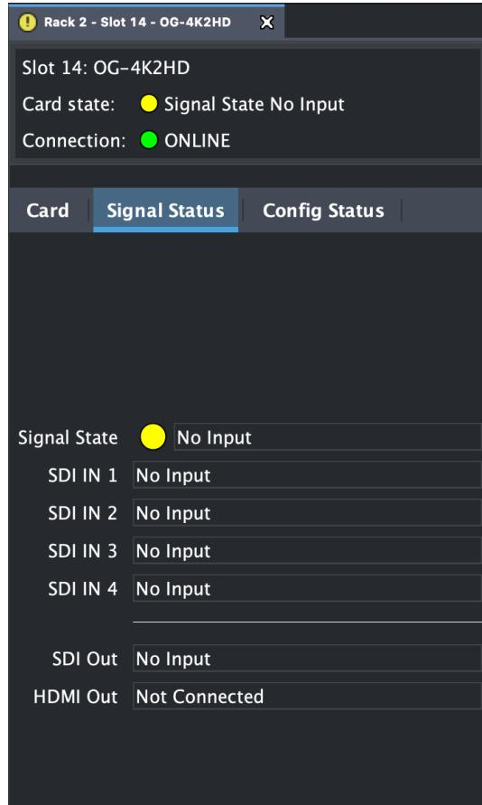
When a signal is present and locked, the DashBoard Control System shows a green Card State and a green Connection under the Signal Status tab. The SDI Signal is also indicated (for example, "1920x1080p59.94 3G-A Quad").
