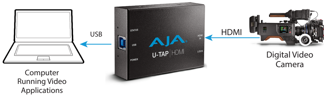
Figure 5. Typical U-TAP HDMI Laptop System Connections
