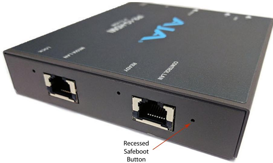
3. While keeping the safeboot button depressed, apply power, then continue holding down the safeboot button for three seconds.
